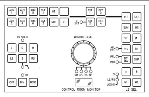
Sets the monitoring and controls the various sources sent to the loudspeakers.
