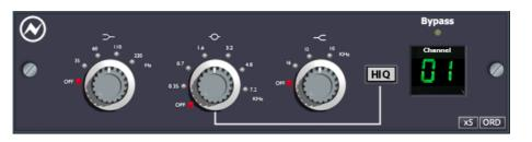
The large green display to the right of the screen indicates which channel number the EQ screen relates to.
