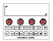
A highlighted/selected track in the DAW will also be shown in the Genesys DAW software screen in the top-right corner in *red LCD type font*, 01, 02... 48. The fader SEL button will also flash to indicate the selected track.
