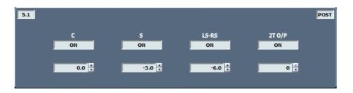
There are individual On/Off controls and +/-10dB of Trim for each of the **C**, **S** and **LS/RS** contributions to the 2T Output, plus a global On/Off and level control ranging from 0dB to  $\infty$  for the 2T Output.
