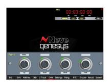
▶ Press **PANS** (the button will light and the screen shown left will open). The encoders now control the Pans.
