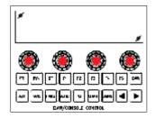
A highlighted/selected track in Logic Pro will also be shown in the Genesys DAW software screen in the top-right corner in *red LCD type font*, 01, 02... 48. The fader SEL button will also flash to indicate the selected track.
