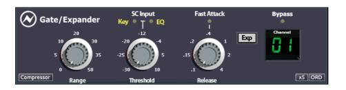
The Gate/Expander controls are accessed by pressing the **DYN** button, and then pressing the  $1^{st}$  encoder to swap the processing screen over to the Gate/Expander view.
