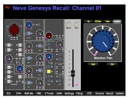
The Channel Strip being displayed on-screen will also be shown on the console surface, with the relevant **SOLO** LED for that Channel strip being lit.
